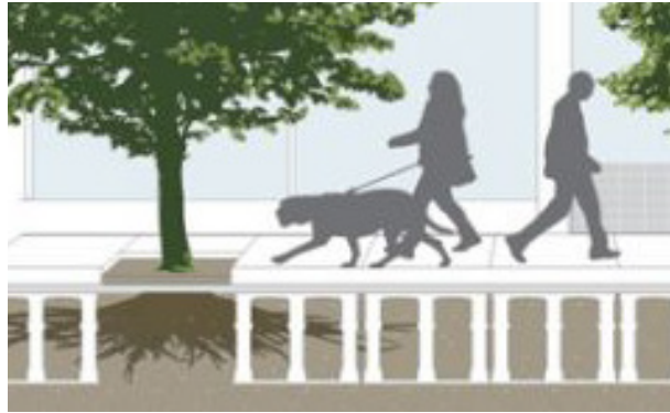
Typical travel zone soil cell section
