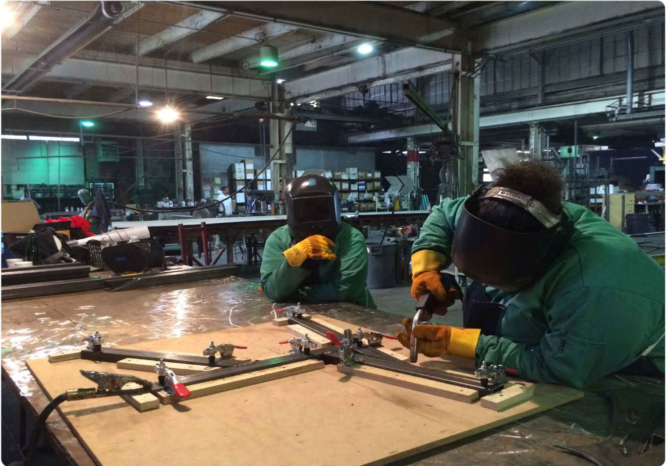
Daniela and EOnka placing steel in the jig
